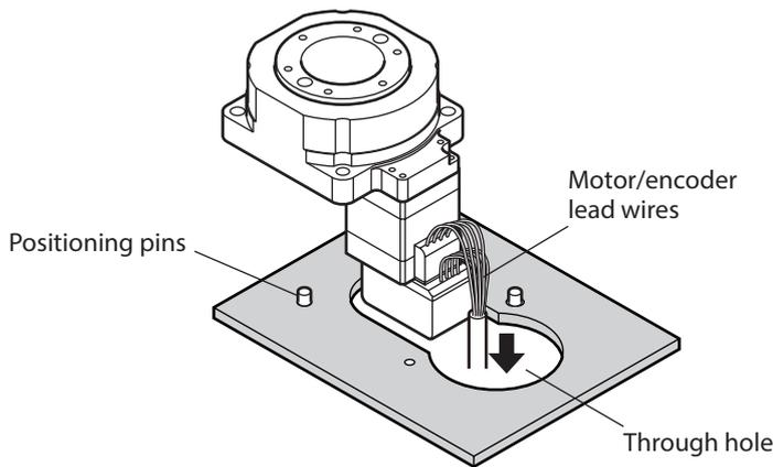
2. Move the actuator to the through hole which diameter is larger, and secure the actuator with screws.
