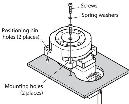
● **When the positioning pin holes are used as mounting holes**
