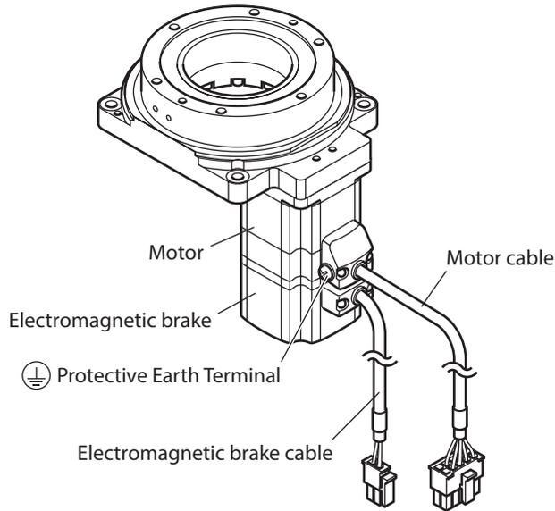
● Actuators equipped with the AZX Series
