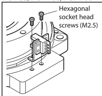
**Note** Do not use the screw holes (M2.5) for the home sensor of the actuator for any other purpose.
