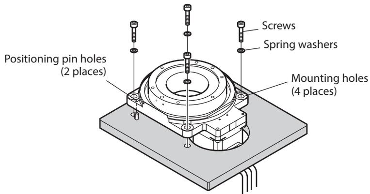
● **Installation procedure: When installing an actuator which cable outlet direction is rightward or leftward**
