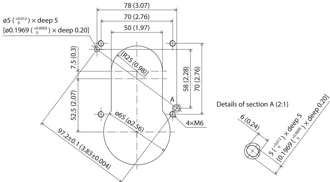
**● Installation procedure: When installing an actuator which cable outlet direction is downward**
