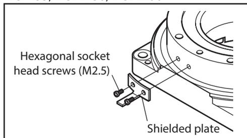
5. In the case of the **DGM60** type, secure the load being attached the shielded plate onto the output table. Machining dimensions of shielded plate for installation (for the **DGM60** type only)
