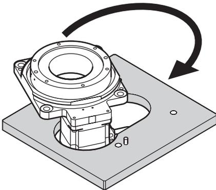
3. Secure the mounting holes with screws (four pieces).
