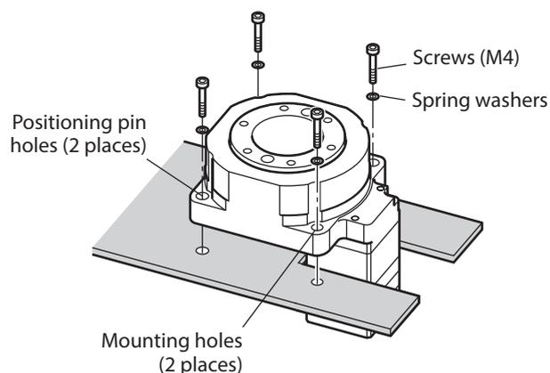
■ **When a mounting plate with through-hole is used**
