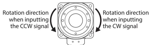
The output table of the actuator equipped with the **AR** Series and the **RKII** Series rotates in the opposite direction as the driver input signal (CW input, CCW input). CW and CCW indicate the rotation direction when viewed from the output table side.
