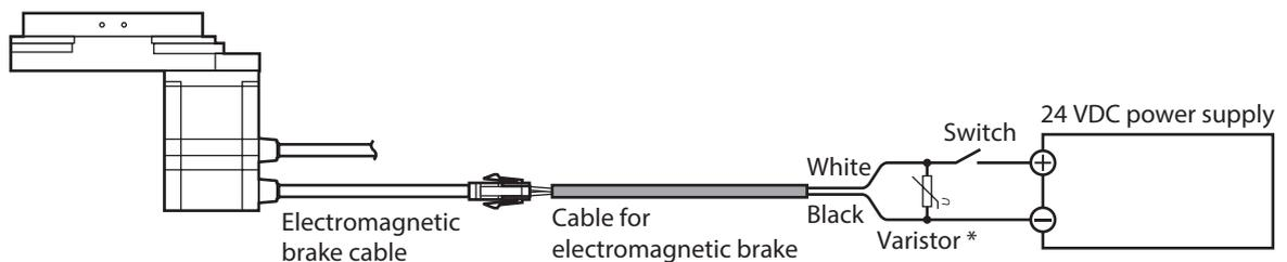
\* Be sure to connect the varistor to protect the contact of the switch or to prevent electrical noise.
