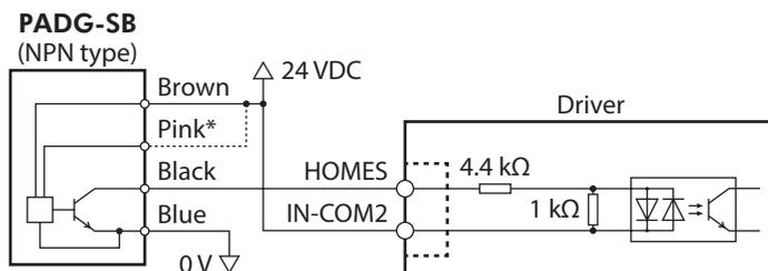
\* The logic of the sensor varies depending on the connection method. When the pink color lead is connected to the brown color lead, the sensor logic will be "normally closed."
