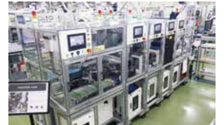
SCARA robots carry out adhesion work on an automated line. Various considerations were taken into account during exterior design, such as using transparent outer panels to make robot operations easy to see.
