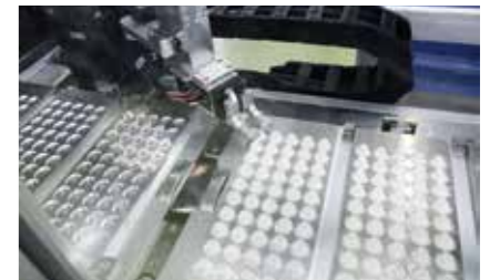
A SCARA robot carries out picking for small components. The gripper current value is controlled to tweak gripping force as needed, which prevents damage to components.
