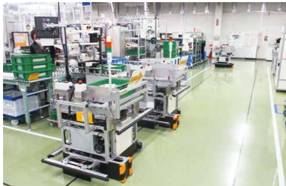
Automated transport of parts, materials and goods between production stages using automatic guided vehicles (AGVs)
