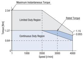
It is the region with a time rating of 30 minutes. Operation for more than 30 minutes may be possible depending on the ambient temperature and heat radiation conditions.
